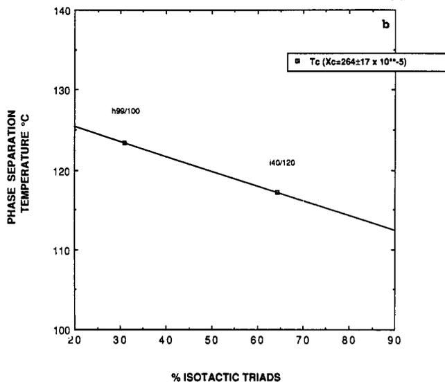
Figure 11. (a) Cloud-point for a 25% PS blend versus percent isotactic triad content of PVME for  $\chi_{c,calcd} = 205 \times 10^{-5} \pm 15 \times 10^{-5}$ . (b) Cloud-point for a 25% PS blend versus percent isotactic triad content of PVME for  $\chi_{c,calcd} = 264 \times 10^{-5} \pm 17 \times 10^{-5}$ .
